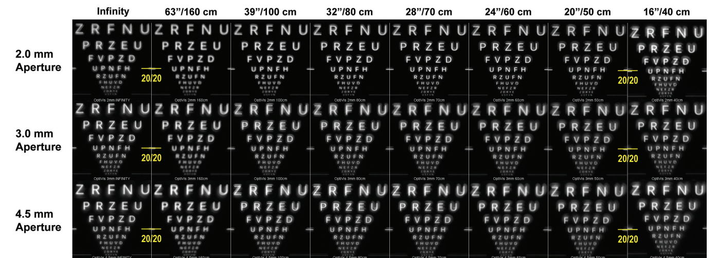
Figure 8: Through focus imagery at 2 mm, 3 mm, and 4.5 mm apertures
